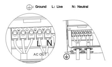
**Note:** The grounding wire shall be as thick as possible (cross-sectional area is not less than 4mm<sup>2</sup>). The grounding point shall be as close as possible to the solar storage inverter. The shorter the grounding wire, the better.
